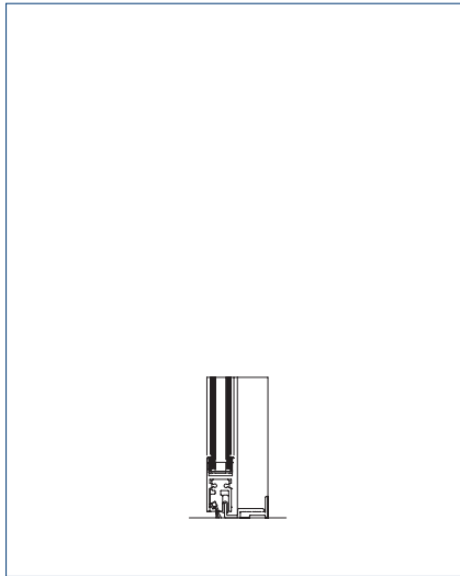
Floor guide: Adjustable for wall installation
